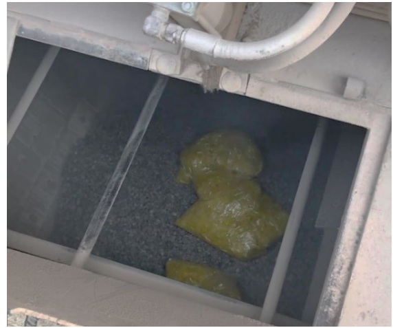
Figure 4: Manual Bag Feed at Batch Plant.
